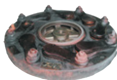
stage valve of a water-cooled compressor after 800 hours
